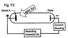
( $\lambda_1$ =420nm) and case 2: red ( $\lambda_2$ =630nm) impinge upon the metal A plate separately to test the currents. If the retarding voltage increases from zero to 10V, please sketch the current reading versus the retarding voltage for case 1 and case 2. In these plots, mark important information that you can obtain from the conditions in this question.
