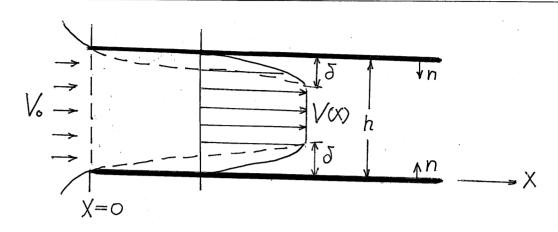
4. (20%)Find the boundary layer thickness  $\delta$ , momentum thickness  $\sigma_2$ , friction drag coefficient  $C_{fL}$  from the Von Kármán integral momentum equation which is
