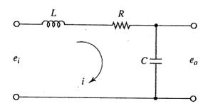
where  $e_i$  is the applied voltage input and  $e_o$  is the voltage output.
