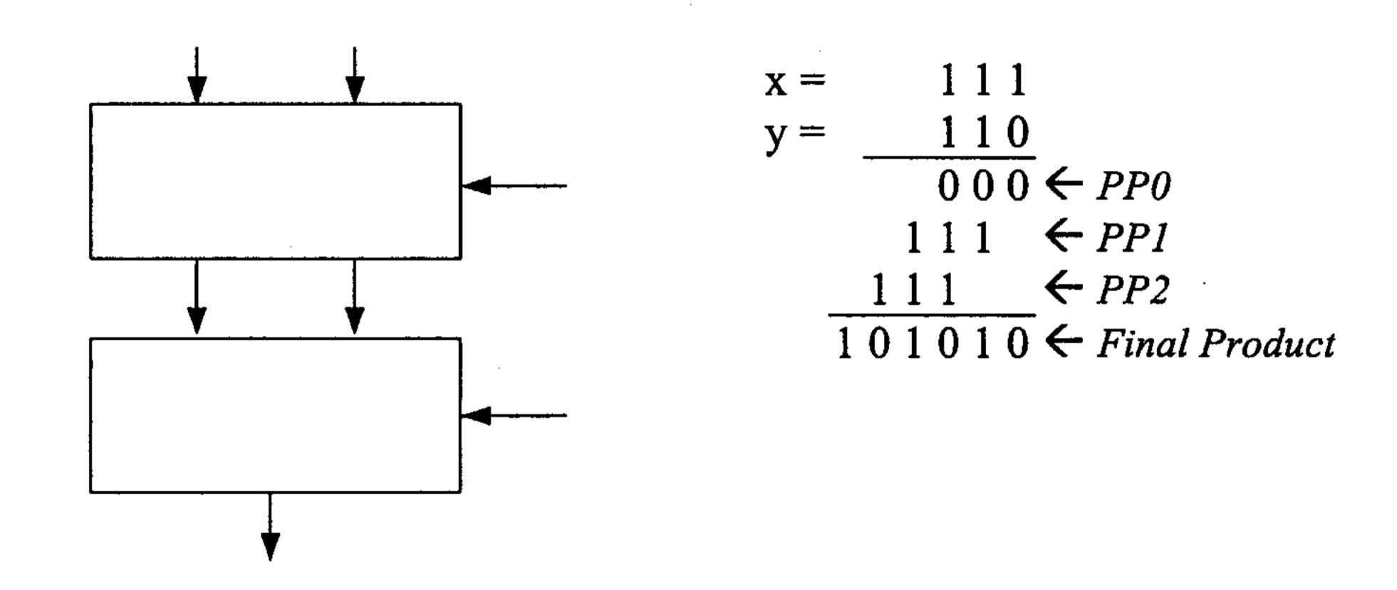
According to the above construction, construct a  $4\times4$  Wallace-tree multiplier using one 7-bit and one 8-bit carry-save adders and one 9-bit parallel adder for a multiplication of (1011)  $\times$  (1110).
