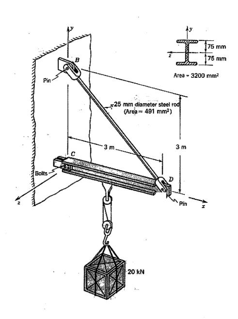
The pulley system in the above figure is located at the midpoint of the beam CD, and Point C can be idealized as a hinge. Answer the following question
