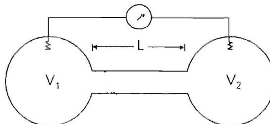
Assume that diffusion may be described by the Fick's first law, that the concentration in each flask is uniform, and that the concentration gradient in the tube is linear. Please derive the following equation and state any other assumptions needed. (12%)
