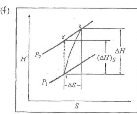
This may interpret the H vs. S diagram of a turbine from state 1 to state 2.
