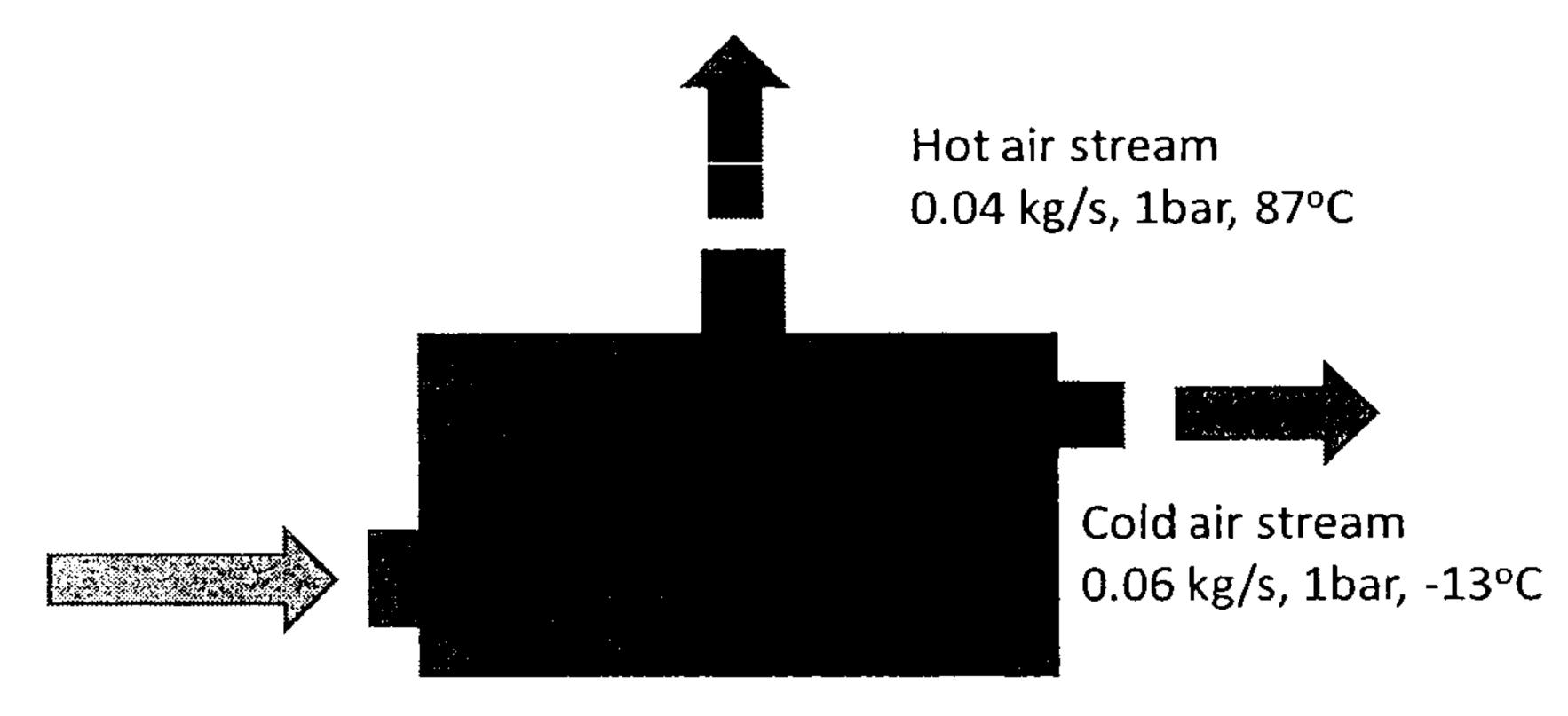
Supplied high pressure air 0.1 kg/s, 1.5bar, 27°C
