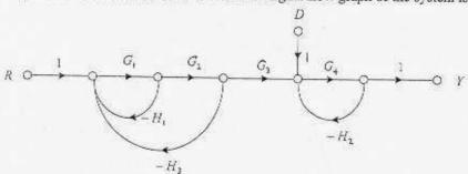
(b) (8%) Let input D = 0, and set system parameters  $G_1 = \frac{1}{s^3}$ ,  $G_2 = \frac{(k-1)}{s}$ ,  $G_3 = 1$ ,  $G_4 = \frac{1}{s^3}$
