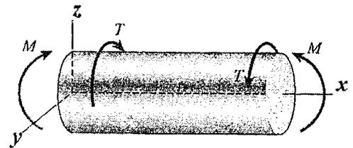
4. (25%) A composite bar of length  $L$  is made of concentric, circular bars bonded together as shown. The shear moduli of elasticity are  $G_c$  and  $G_t$  respectively for the core and the tube, and the polar moments of inertia for the core and the tube are  $J_c$  and  $J_t$ , respectively. Consider that the composite bar is acted upon by a total torque  $T$ .
