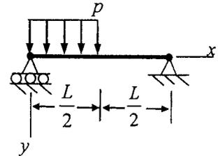
2. (25%) A uniform load of intensity  $p$  is acting on the beam of flexural rigidity  $EI$  as shown. By solving the beam equation, determine (a) the equation of the deflection curve, and (b) the support reactions at  $A$  and  $B$  for the beam.
