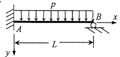
The beam equation is given as  $EI \frac{d^4 y}{dx^4} = p$  or  $EI \frac{d^2 y}{dx^2} = -M$ .
