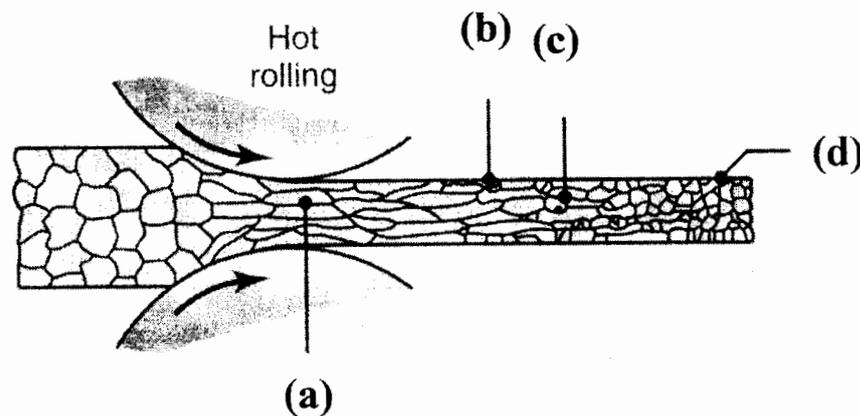
Figure A Microstructure change in hot rolling
