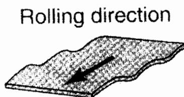
Figure B Defect in sheet metal rolling
