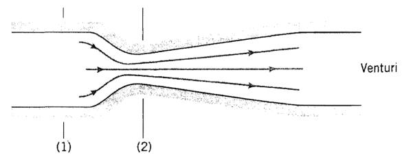
Show that the flow rate for a fluid going down the tube is
