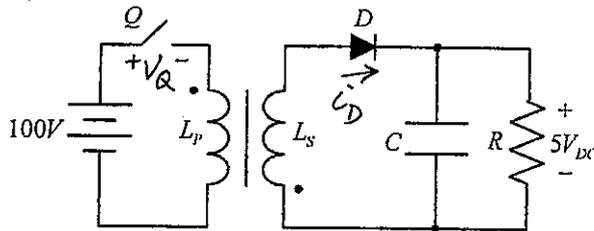
Given:  $L_p=200 \mu\text{H}$ ,  $L_s=20 \mu\text{H}$ ,  $C=100 \mu\text{F}$
