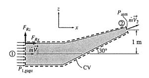
Determine (a) the pressure at the inlet and (b) the anchoring force needed to hold the elbow in place.
