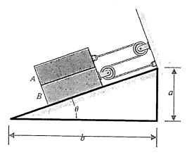
2. Determine force P on the cable if the spring is compressed 0.05 m when the mechanism is in the position shown. The spring has a stiffness of k = 600 N/m. (25%)
