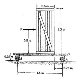
2. The coefficient of static friction between the 150-kg crate and the ground is  $\mu_{\rm s}$  = 0.3, while the coefficient of static friction between the 80-kg man's shoes and the ground is not known. Determine the minimum coefficient of static friction between the man's shoes and the ground so that the man can move the crate. [25]
