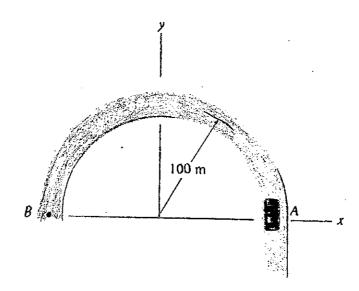
4. The sports car, having a mass of 1700 kg, is traveling horizontally along a 20° banked track which is circular and has a radius of curvature of  $\rho$  = 100 m. If the coefficient of static friction between the tires and the road is  $\mu_s$  = 0.2, determine the minimum speed at which the car can travel around the track without sliding down the slope. [25]
