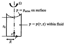
Cylindrical coordinates are appropriate for this problem, and the equations of motion are given
