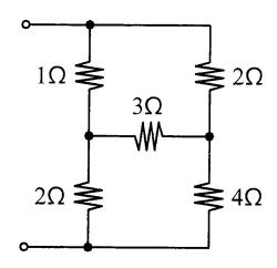
2. Set node 4 as the reference ground. Also, set the node voltage of node 1 as  $v_1$ , the node voltage of node 2 as  $v_2$ , and the node voltage of node 3 as  $v_3$ . Use node method and write a complete set of equations that solve the voltages  $v_1$ ,  $v_2$ , and  $v_3$  (5%)
