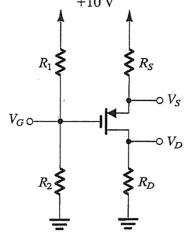
7. Consider the FET amplifier of the following Figure for the case,  $V_t = 2 \text{ V}$ ,  $k'_n(W/L) = 1.0 \text{ mA/V}^2$ ,  $V_{GS} = 4 \text{ V}$ ,  $V_{DD} = 10 \text{ V}$ , and  $R_D = 3.6 \text{ k}\Omega$ . (12%)
