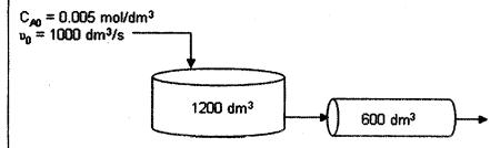
If the volume of the CSTR is 1200 dm<sup>3</sup> and the tubular reactor volume is 600 dm<sup>3</sup>, what are the intermediate and final conversions that can be achieved with the existing system? The reciprocal rate is plotted in the figure below as a function of conversion for the conditions at which the reaction is to be carried out.
