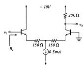
4. The two transistor amplifiers shown in the following figure combine an FET and a BJT to achieve both a high input impedance and a large voltage gain. Determine the voltage gain  $V_0/V_i$  of the amplifier by considering  $Q_i$  with  $g_m=1ms$ ,  $r_\pi=1k\Omega$  and  $\beta=120$ . (20%)
