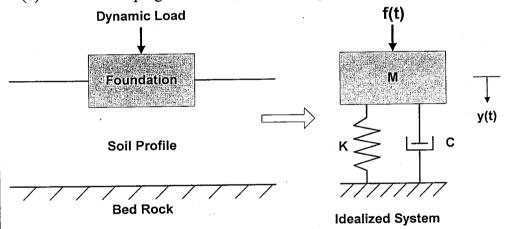
3. The above idealized system has an **impulse response**  $h(t) = e^{-t}$ . Assume the initial conditions y(0)=y'(0)=0. Find the response y(t) for the applied force f(t) as shown below. (10%)
