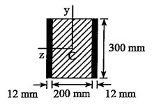
3. Determine the distances  $e_y$  and  $e_z$  to locate the shear center S of the following 2 thin-walled beams with uniform thickness t as shown. (20%)
