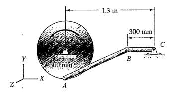
6. A thin-walled cylinder held in position by a cord AB. The cylinder has a mass of 10 kg and has an outside diameter of 600 mm. What are the normal and friction forces at the contact point C at the instant that cord AB is cut? Assume that no slipping occurs. (15%)
