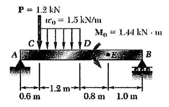
6. (20pts) Also use the figure above, determine the deflection at the midpoint D ( E = 200 GPa and  $I = 6.87 \times 10^{-6}$  m<sup>4</sup>).
