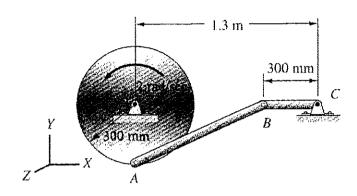
4. A stepped cylinder having a radius of gyration k = .40 m and a mass of 200 kg is shown. The cylinder supports a weight W of mass 100 kg with an inextensible cord and is restrained by a linear spring whose constant K is 2 N/mm. What is the angular acceleration of the stepped cylinder when it has rotated 10° after it is released from a state of rest? The spring is initially unstretched. What are the supporting forces at this time? (25%)
