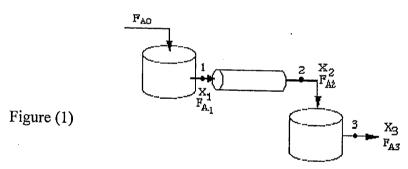
5. [20%] The adiabatic exothermic irreversible gas-phase reaction  $2A + B \rightarrow 2C$  is to be carried out in a flow reactor for an equimolar feed of A and B.
