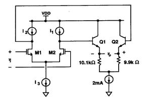
6. [10%] Consider the circuit shown below. Assume that all the MOSFETs are operated in the saturation region,  $V_{Tn} = |V_{Tp}| = 0.5V$ , If the transconductance of M1, M2, M3, and M4 = 1mA/V. The transconductance
