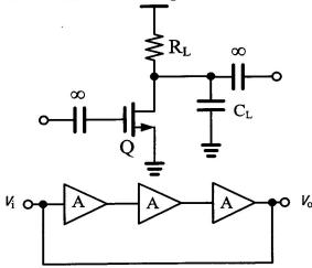
(a) (10%) What is the g<sub>m</sub> value such that the feedback circuit oscillates? What is the oscillation frequency?
