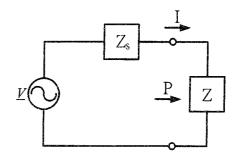
5. The circuit shown below is the frequency domain model for the output of an amplifier operating at  $\omega$ =10<sup>5</sup>. The load has a fixed resistance of 500  $\Omega$ . Identify the load reactance X and the transformer's turn ratio N to achieve the maximum power transfer. Assume that the transformer is an ideal transformer. (20%)
