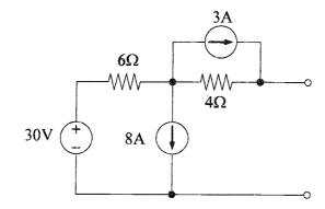
2. Find the values of  $v_1$  and  $i_a$  in the circuit shown below. (20%)
