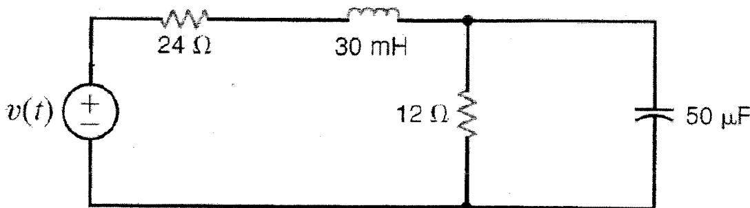
4. Find the Z parameters for the two-port network in the following figure.
