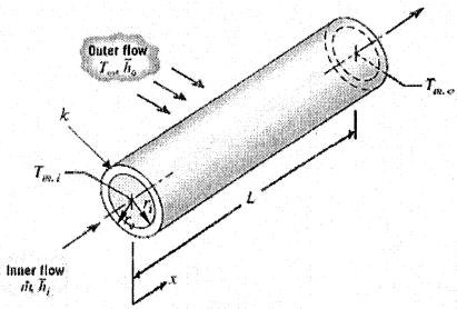
show that the heat transfer rate (q) between the outer fluid and inner fluid is
