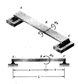
3. An alumina beam specimen is to be tested in a four-point bending test rig, as shown in the figure below. The specimen has a rectangular cross section with the dimensions b = 1.2 mm and h = 1.8 mm.
