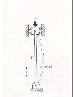
Figure 1. Column buckling.
