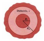
2. Consider a very long coaxial cable. The inner conductor has a radius a and is maintained at a potential  $V_0$ . The outer conductor has an inner radius b and is grounded. Determine the potential distribution in the space between the conductors. (20 points)
