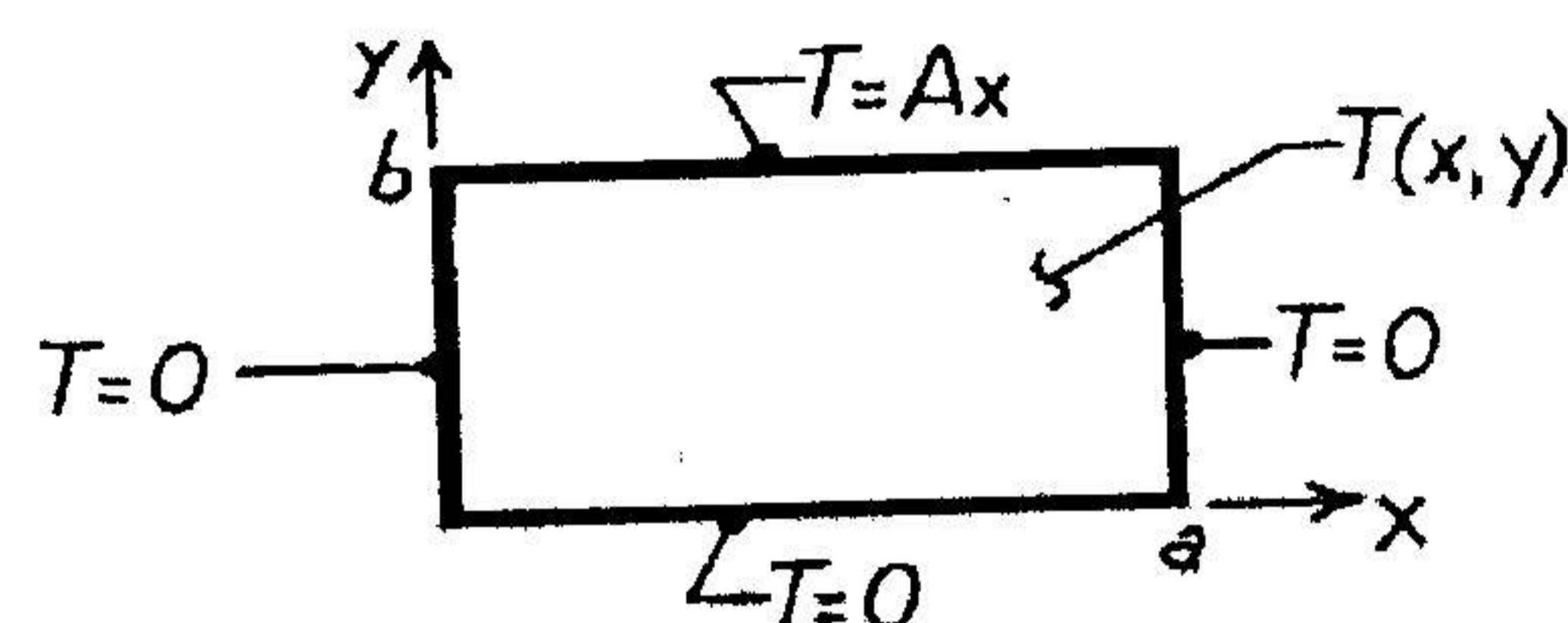
Steady state, 2D, constant properties conduction heat transfer problem.
