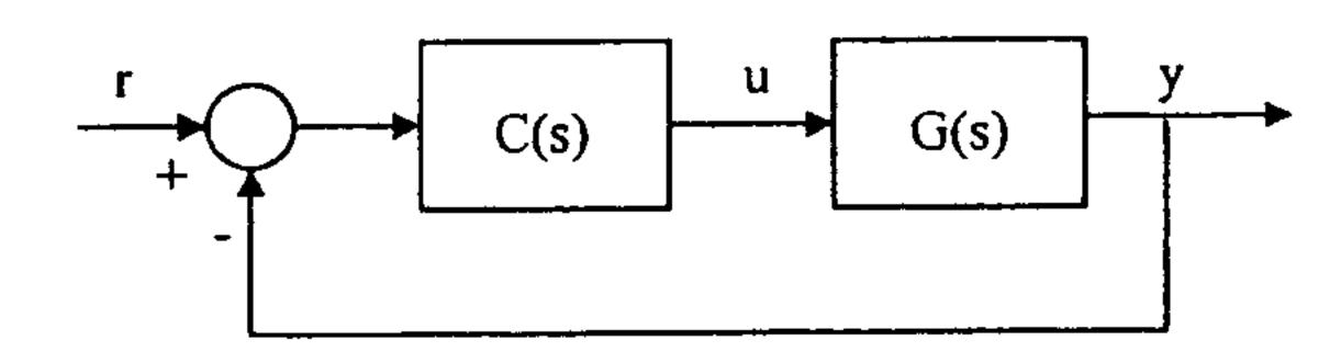
If the controller C(s) is of proportional type (i.e. C(s)=K, a constant), find the range of K so that the closed-loop system is stable. (7%)
