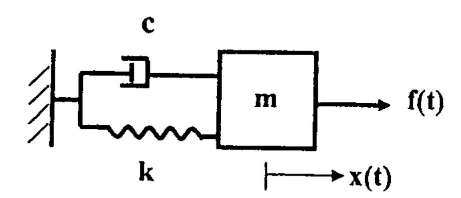
(a) Draw a free body diagram (FBD) of mass m for arbitrary displacement x(t) and show that the equation of motion:
